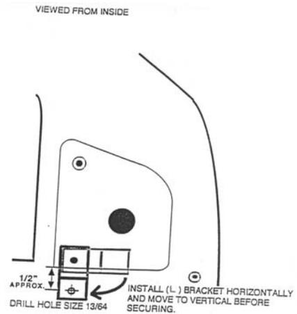
7. The other end of the "L" bracket is to be attached to the interior door frame post with the self-tapping screw provided (see diagram below). Drilling a small hole in the interior frame post will be necessary, the hole size must be 13/64" and as close as possible to the center of the end of the "L" bracket.
